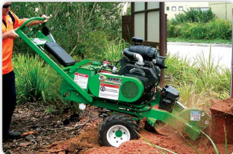
Oversize bearings in the pump handle the shock loads from stump grinding, while an economical 27-horsepower engine powers the hydraulic systems and self-propelled undercarriage. The cutter wheel has a class leading 50 inch (127cm) swing arc that can also grind to a depth of over 12 inch (30cm), and at just 700kg it's one of the lightest four-wheeled, self-propelled stump grinders available.
