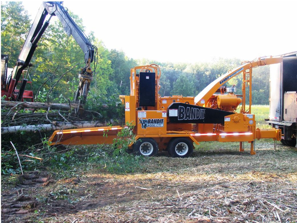
Padgette Logging, based in North Carolina USA, invested in Bandit’s Model 2590 whole tree chipper to produce a ¾” chip and is thrilled with the results
