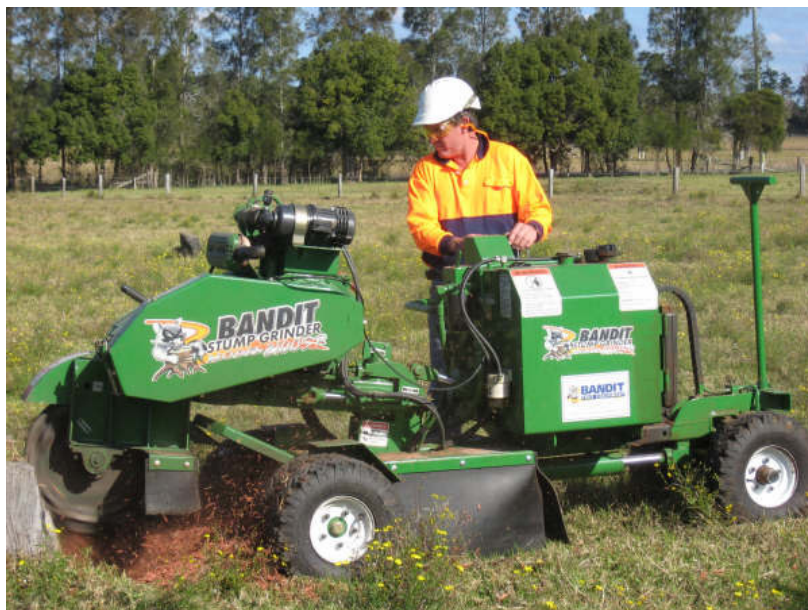
Steve Jeskie from Macleay Valley All Terrain Tractor with his Bandit Model 2100 diesel grinder
